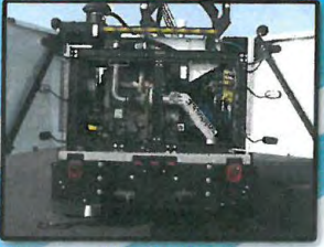
The powerful 115 HP John Deere Tier 2 diesel auxiliary engine is located at the rear of the sweeper, reducing cab noise and heat, while also allowing easy access and ground level service.
