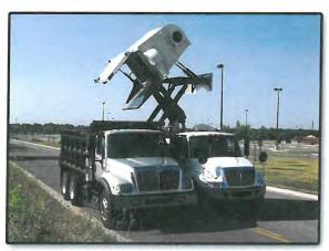
The TYMCO Model 500x\* has a large stainless steel discharge chute, which projects debris into the middle of the container without the need of a side shift. The chute is designed to float 45 degrees upward, preventing major damage should it come in contact with the debris container.
