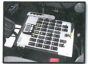
In cab controls are center mounted and illuminated for ease of operation from either driving position.
