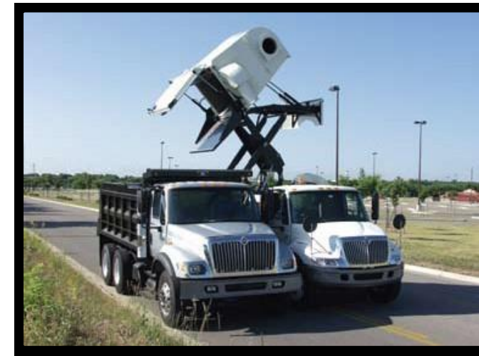
The TYMCO Model 500x ® has a large stainless steel discharge chute, which projects debris into the middle of the container without the need of a side shift. The chute is designed to float 45 degrees upward, preventing major damage should it come in contact with the debris container.
