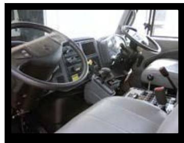
The operator friendly cab features dual steering with tilt and dual instrumentation.
