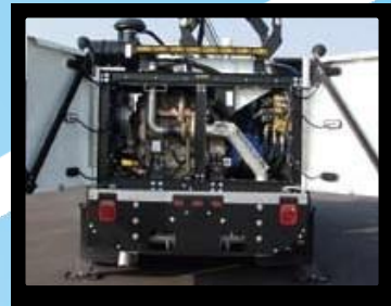
The Tier 2 diesel auxiliary engine is located at the rear of the sweeper, reducing cab noise and heat, while also allowing easy access and ground level service.
