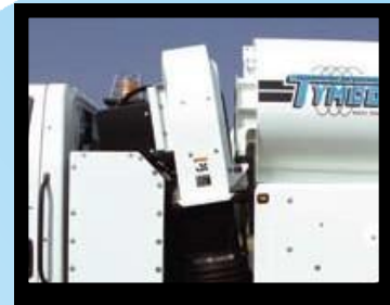
The Tilt-N-Seal ® blower system ensures long seal life between the hopper and blower housing.
