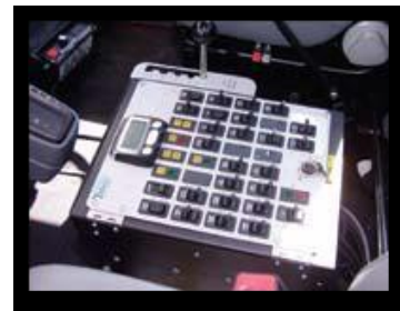
The cab controls are center mounted and illuminated for ease of operation from either driving position.
