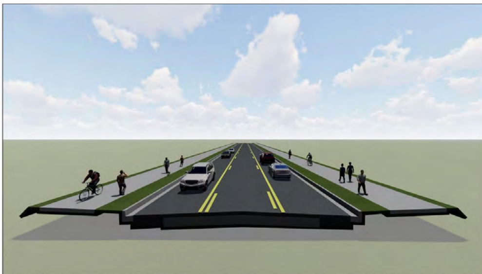
Typical Section B Shared-use path* *Shared-use path may be on one or both sides of the roadway.*
