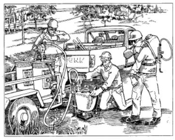
Figure 9. An interlocking valve connection between fill hose and backpack is preferred.
