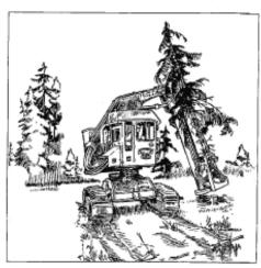
Figure 5. Feller-buncher.
