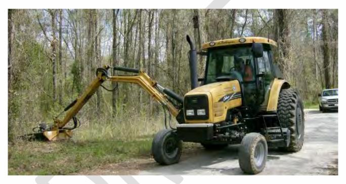
Slope mower cutting County right-of-way
