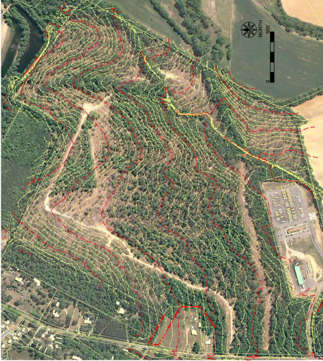
Aerial Map photo from Richland County GIS web site 11/2005 with 2' Survey Contours overlaid
