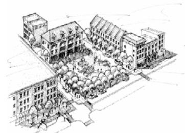
An "outdoor room" is created by surrounding an open plaza or greenspace with buildings.
